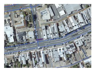
The width of the road would allow for a refuge to help cross the 11.5m width road. It would also assist in preventing vehicles cutting the corner and turn properly onto Ingor from Barkly
